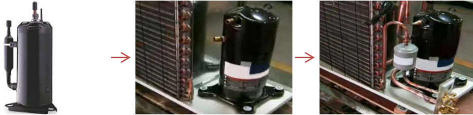
Fig. 5.2.6: Assembling of the compressor unit
