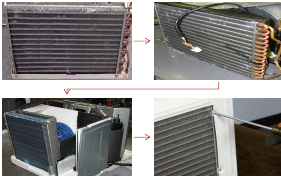
Fig. 5.2.5: Assembling of the evaporator unit
