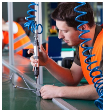
Fig. 4.1.2: Pneumatic tool used in RAC components' assembling
